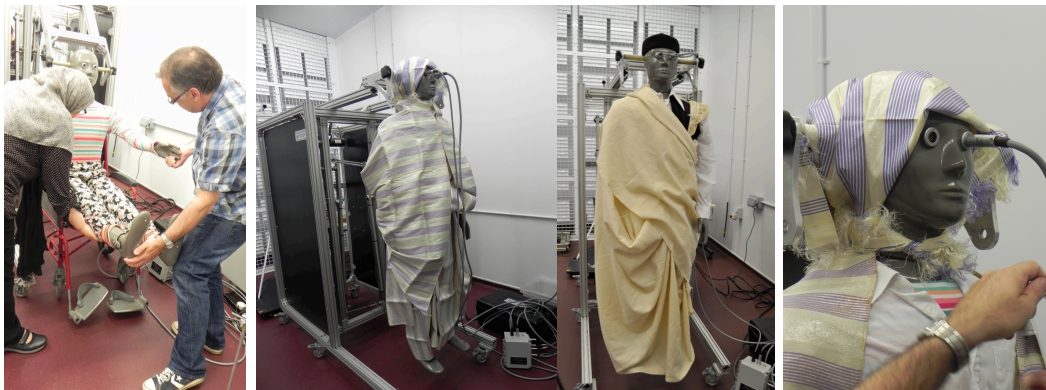
Figure (5.3) the traditional Libyan cloth for female and male worn on the thermal manikin Newton
